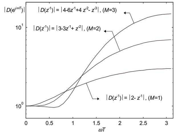
Fig. 4. Frequency characteristics of Newton's predictive filter for  $p = 1$  and  $M = 1, 2$  and  $3$
