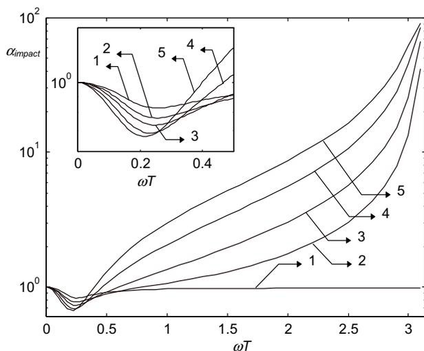
Fig. 9. Frequency characteristics of complementary sensitivity function of IMPACT structure with (1) prediction polynomial and (2) with LSN predictor having: (2)  $T_f = 0.05$ , (3)  $T_f = 0.1$ , (4)  $T_f = 0.2$ , and (5)  $T_f = 0.33$ .
